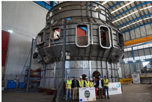
JT-60SA Cryostat Vessel Body Integral Preassembly at Factory
